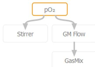
The parameters *Stirrer* and *GM Flow* are activated at the same time to control the  $pO_2$  parameter. The *GasMix* parameter is only activated when the setpoint of the  $pO_2$  parameter has not been achieved by the *Stirrer* and the *GM Flow*.
