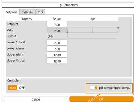
In the pH measurement system with analog pH sensor, the *pH* parameter has the additional function *pH temperature comp.* (pH temperature compensation). In the digital pH measurement system, this function is integrated into the pH sensor. The pH temperature compensation must be activated during a cultivation so that temperature compensated values can be generated. That is, this is used to correct the temperature dependence of the measurement principle.
