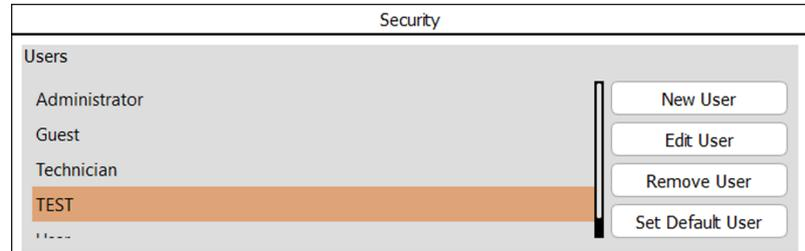
2. Select the desired user (here: *TEST*) from the selection list and press **Remove User**.
