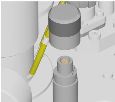
3. → Manually remove the steel cap from the sensor head connection.
