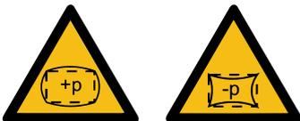
The vessel may be pressurized. Incorrect manipulation or exceeding the permissible working pressure can cause built-in-parts to be flung away. This can result in liquids and gases being expelled at high pressure.
