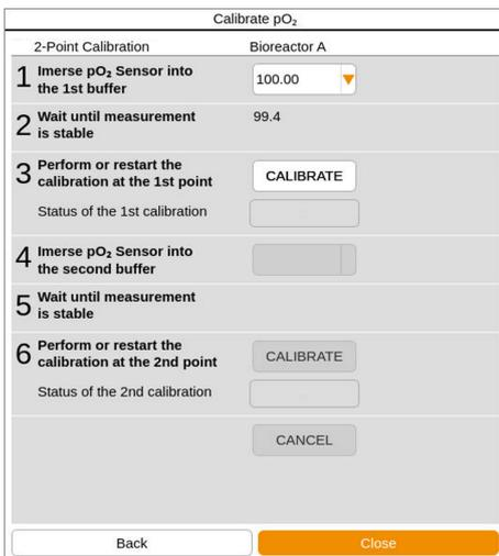
The calibration process can be continued from the last saved point at any time, if the menu was closed using **Close**. However, this does not apply if another calibration process is started.
