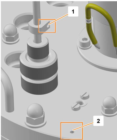
1. ➔ Plug the red banana plug of the sensor cable into the side connection (1) of the antifoam sensor.
