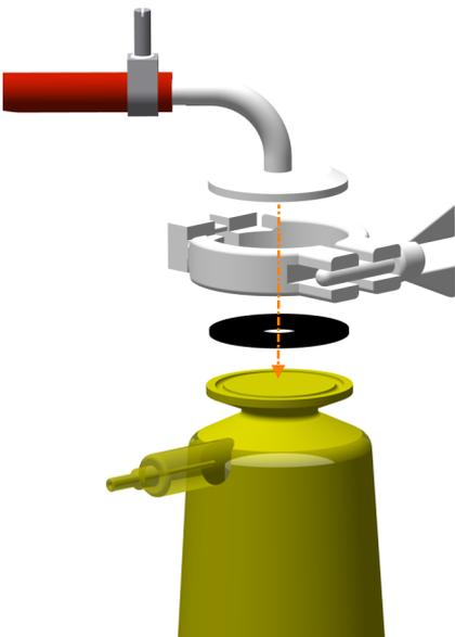
3. → Place the flat gasket and flange of the exit gas hose flush on the flange of the exit gas filter and affix them with a clamp.
