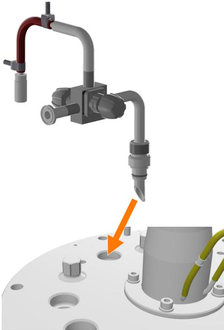
1. → Insert the connection nozzle of the block valve *13.16.01* / *13.16.03* into a 19 mm port in the vessel top plate and tighten manually.
