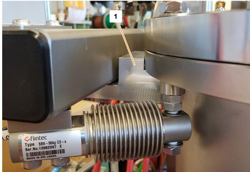
The safety plates prevent the load from being applied to the load cells by the vessel. The safety plates are only removed when qualified personnel installs the device and are handed over for safekeeping. The transportation safety device must be mounted prior to any transport of the device.
