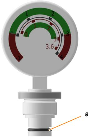
The maximum permissible vessel pressure is 3.0 bar. Manometer *08.30.01* indicates the pressure in the vessel in a range from 0 bar to 4.0 bar. The manometer has two different measuring scales. The outer scale corresponds to the pressure at a vessel temperature of 25 °C. The inner scale corresponds to the pressure at a vessel temperature of 121 °C. Two red markings indicate the non-permissible pressure range of the vessel.
