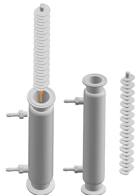
5. → Carefully remove the baffle body from the exit gas cooler.
