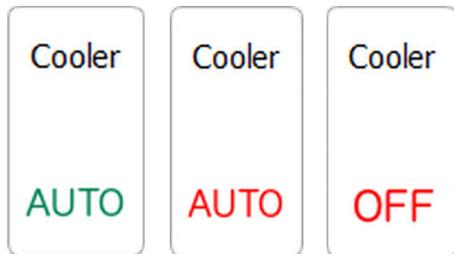
The **Cooler** button signals the *01.06.06* valve for the water feed to the exit gas cooler. In automatic mode, the valve opens during an running cultivation and during full sterilization it opens in the cool down phase. For a manually switched valve, no water can be fed in, the valve remains closed. This is signalized with *OFF* in a red font.
