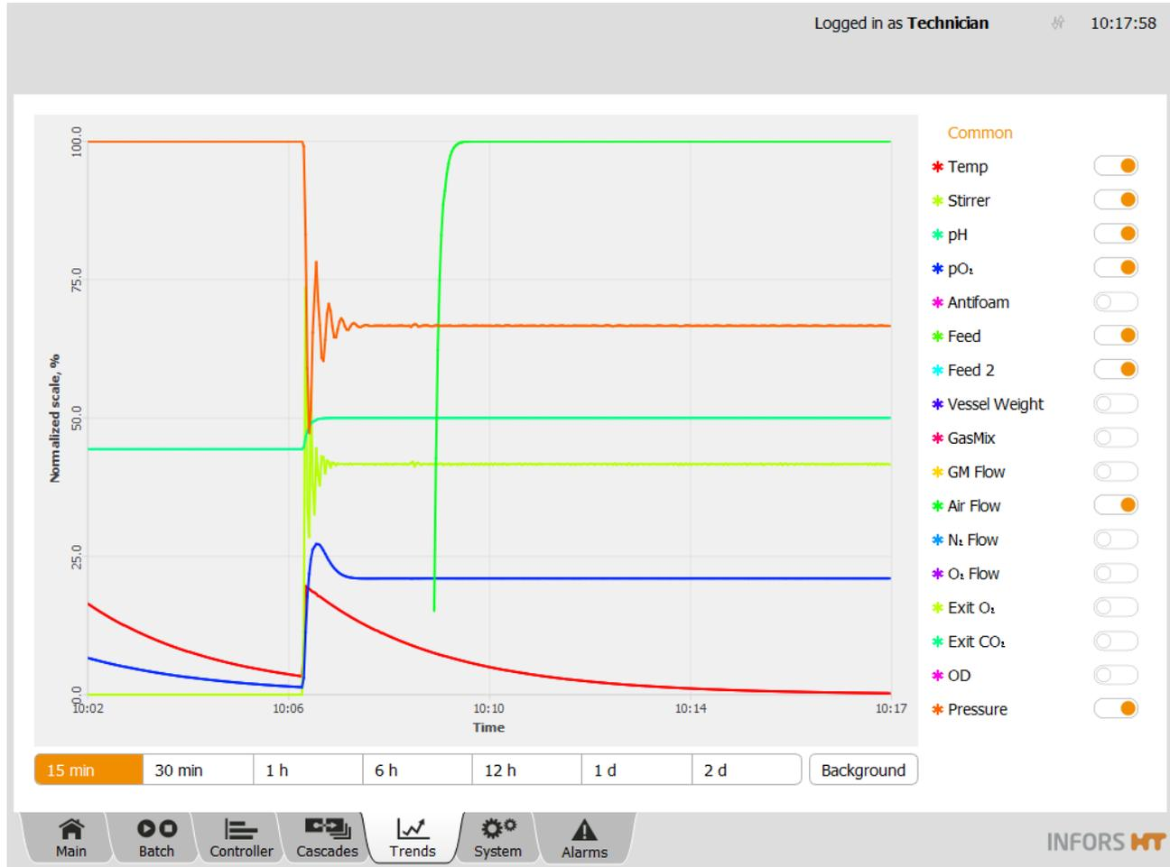
The touch screen operating panel keeps the actual values of the parameters in a buffer memory and displays them continuously as a diagram in the *Trends* main menu. This data cannot be archived, edited or exported. However, this data can be transferred to a computer connected via a network, for example, by using eve®, and then be archived there.
