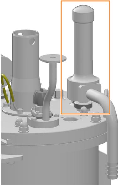
The safety valve mounted on the vessel top plate with lifting device protects the bioreactor vessel (not the vessel jacket) against an inadmissible overpressure. It must be mounted and intact at all times.
