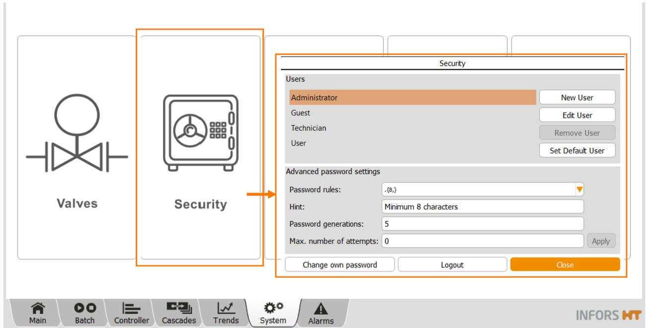
The *Security* submenu is used for logging on and off to and from the system. Users can also be added or deleted here, passwords can be set and access rights can be assigned. The number of functions available depends on the authorisation of the user that is logged on:
