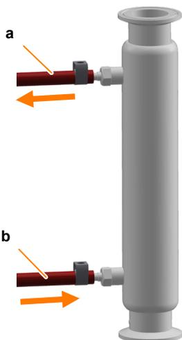
The exit gas cooler dries the exit gas through condensation, thus preventing the exit gas filter from becoming clogged with moisture. At the same time, it also prevents water loss in the culture medium.
