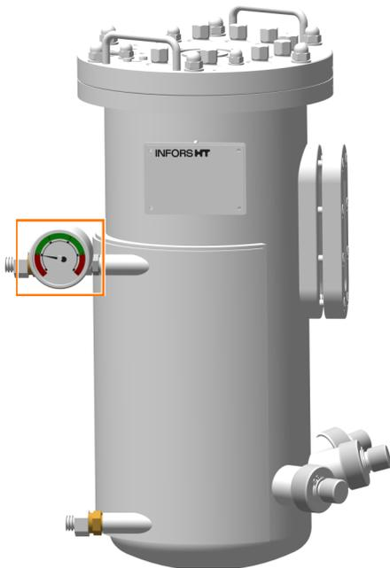
The maximum permissible pressure in the temperature control system is 3.0 bar. The manometer 01.30.01 installed on the water outlet of the vessel jacket indicates the pressure in a range from -1.0 bar to +4.0 bar.
