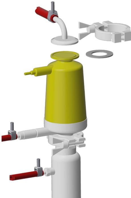
1. → Remove the clamp between the exit gas filter and the exit gas hose.
