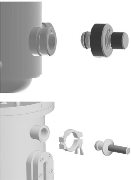
**i** If the device is to be used with the (optional) mobile CIP unit of the device manufacturer, an adjusted vessel design is required. In this case, the vessel has two additional Tri-clamp ports with blanking plugs.
