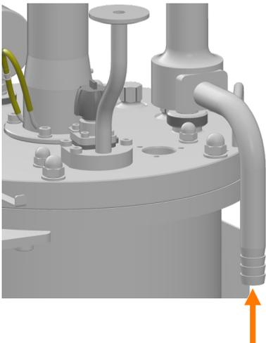
2. → Ensure that the provider-side hose or piping is connected to the overpressure venting pipe; connect if necessary.
