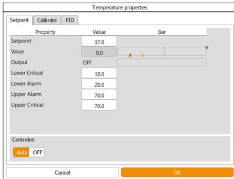
Controlled process parameters and their actual values are displayed in the form of buttons. Pressing the button of a parameter leads to the parameter options. Example on the left: *Temperature* parameter, *Setpoint* option.
