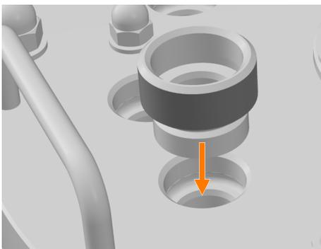
3. → Manually screw the antifoam sensor into the septum collar.
