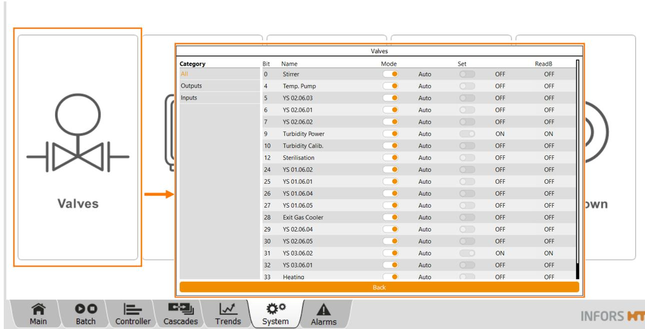
The submenu *Valves* displays the digital outputs and inputs of the control board. The overview is predominantly used for fault diagnosis. All valves and digital outputs are set to automatic mode (*Auto*) ex-factory. These settings must not be changed! The view of all (*All*) digital inputs and outputs or only the display of the inputs or outputs can be selected in column (*Category*). The main column contains:
