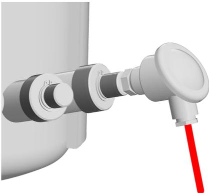
2. ➔ Manually tighten the coupling nut clockwise and straighten the sensor at the same time.
