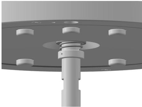
The mechanical seal must always be lubricated. For this purpose, there are two connection nozzles with a silicone hose on the drive hub (→ Chapter 2.7.3 'Lubricating the Mechanical Seal' on page 54).
