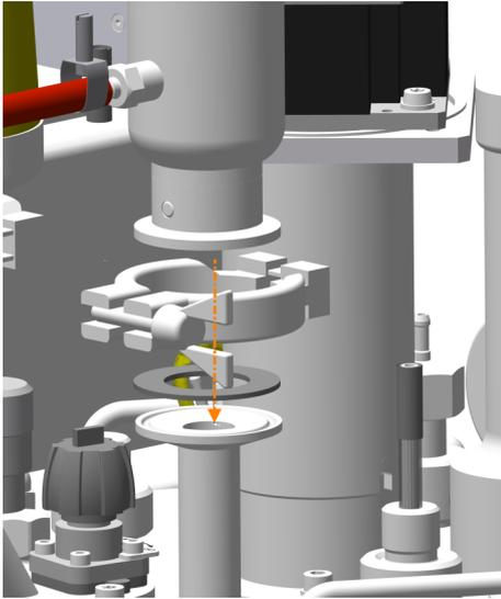
2. → Place the flat gasket and exit gas cooler flush on the flange on the vessel top plate and secure them with a clamp.
