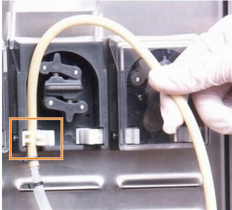
**4.** → Thread the pump hose around the pump head and push in gently.
