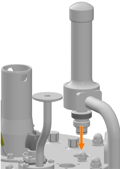
1. → Insert the safety valve with O-ring into the 19 mm port and screw it in by hand.
