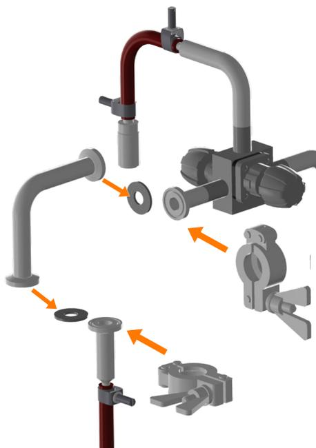
2. → Use the clamps to connect the condensate elbow to block valve *13.16.01* / *13.16.03* and connect to the condensate line.
