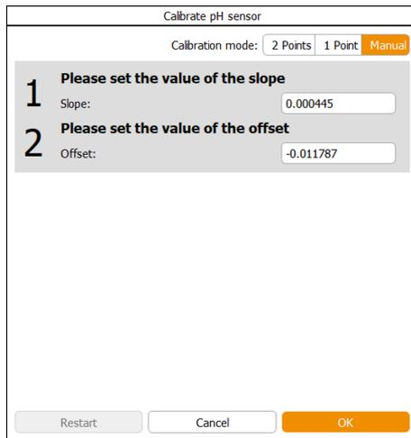
3. → Depending on the difference between the two pH measurements, either add the result to the displayed "Offset" or subtract it and enter it.
