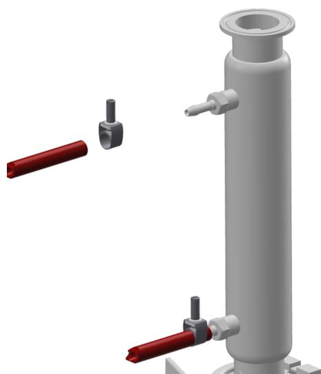
3. → Remove the hose clamps and disconnect the red pressure hoses for water inlet and outlet from the exit gas cooler.
