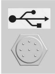
1. ➤ Connect the special cable supplied by the device manufacturer to the connection socket on the back of the operating panel and connect the USB stick.
