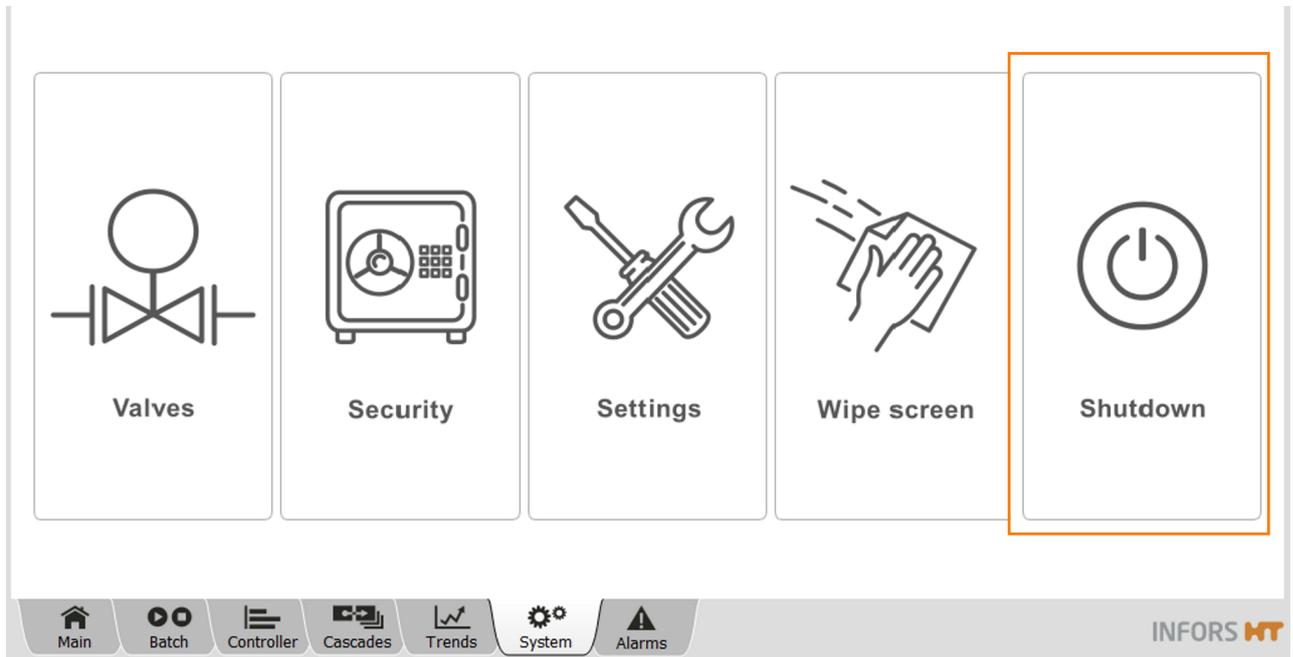
The *Shutdown* submenu has only one function: it shuts down the system. This is only possible when all processes have stopped.
