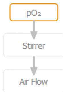
The *Stirrer* parameter is activated as the first one in the cascade to control the  $pO_2$  parameter. The *Air Flow* parameter is only activated when the setpoint of the  $pO_2$  parameter has not been achieved by the *Stirrer*.
