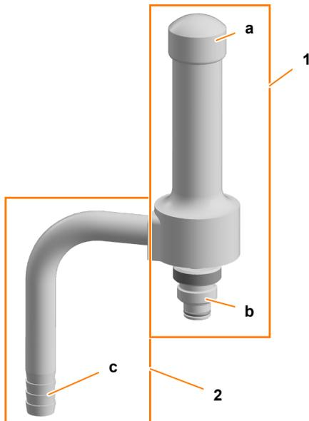
The safety valve has a connection thread for mounting in the 19 mm port in the vessel top plate. It also has a short overpressure venting pipe.
