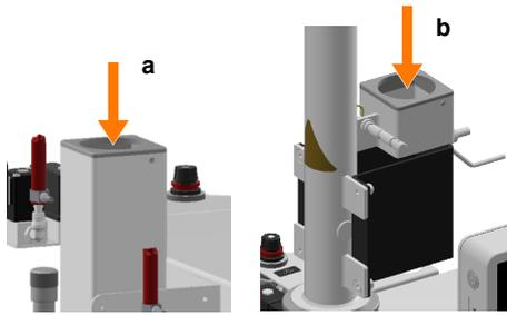
2. → Place the motor in the holder of the lifting device on the central column (a) or (if available) into the holder for the vessel top plate (b).
