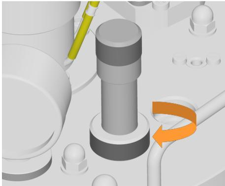
2. → Carefully insert the pressure sensor with O-ring into the 19 mm port and tighten the hollow screw by hand.
