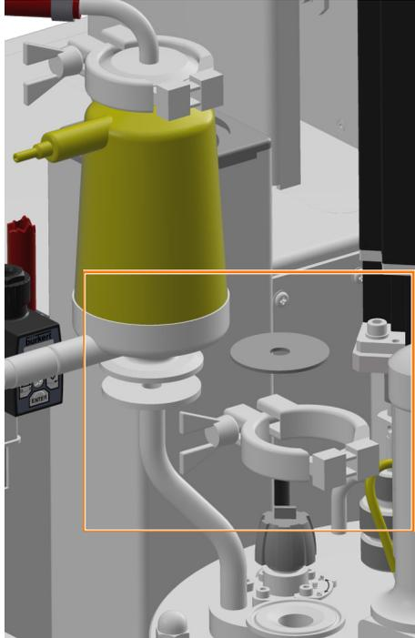
1. ➔ Remove the clamp between the inlet air filter and connection flange on the vessel top plate.
