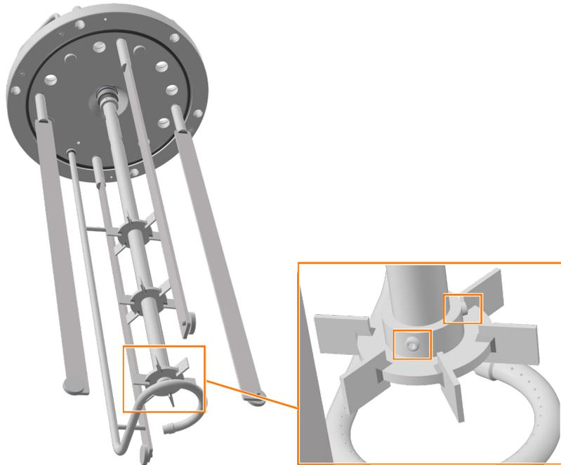
Depending on the vessel size, two (15 L TV) or three (30 L and 42 L TV) Rushton impellers are affixed to the stirrer shaft using grub screws.
