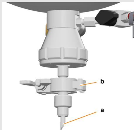
This valve type has a needle (a) for sampling. The inlet air filter is connected to the flange on the harvest/sample valve with a clamp (b) and a flat gasket. For sampling, the steam trap must be unscrewed from the needle.
