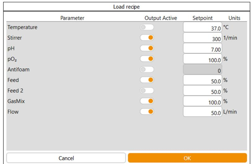
Here, all parameters used in the recipe are listed. Setpoints can be changed subsequently and parameters can be activated or deactivated. Use **OK** to start the cultivation.
