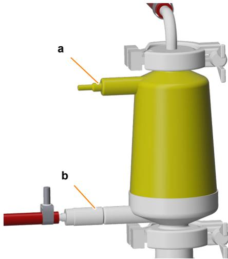
A steam sterilizable membrane filter is used as the exit gas filter. The filter has two manual twist valves. The condensate hose is connected to the lower twist valve (b). This valve must be open. The upper twist valve (a) is not used and must be closed.
