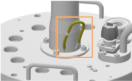
To ensure lubrication of the mechanical seal, the silicone hose at the bottom of the drive hub of the top plate must always be filled with liquid (glycerine).
