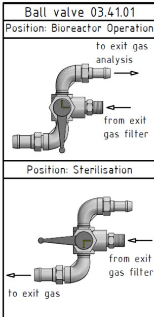
During cultivation, exit gas is routed through the gas sensors. During sterilization, it must be discharged directly into the provider's exit gas line to protect the sensors from moisture. The operator manually makes this switch using the 3-way ball valve 03.41.01.
