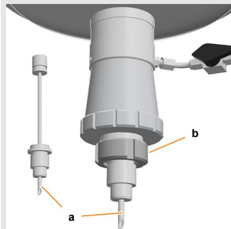
This valve type has a valve insert with a needle (a) for sampling. The valve insert is placed in the harvest/sample valve and affixed using a groove nut (b). For sampling, the steam trap must be unscrewed from the valve insert with needle.
