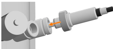
**2.** → Insert the sensor into the Ingold nozzles and tighten it manually using the coupling nut.
