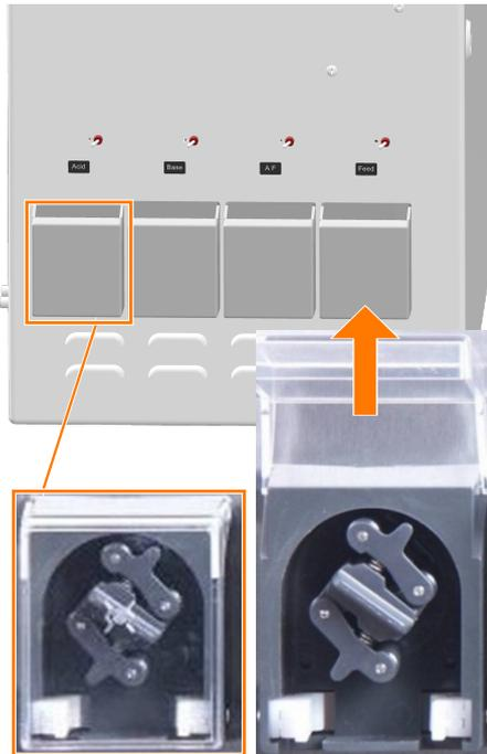
By default, the lower part of the instrumentation cabinet features four peristaltic pumps with hinged cover. The pumps are driven by stepper motors and run clockwise in automatic operation. The pumps are labelled from left to right according to their function:
