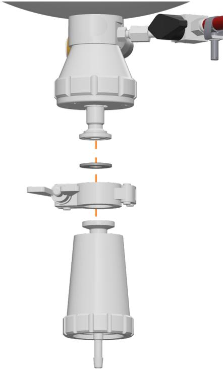
1. Open the clamp and remove the steam trap with the flat gasket from the connection flange of the harvest/sample valve.
