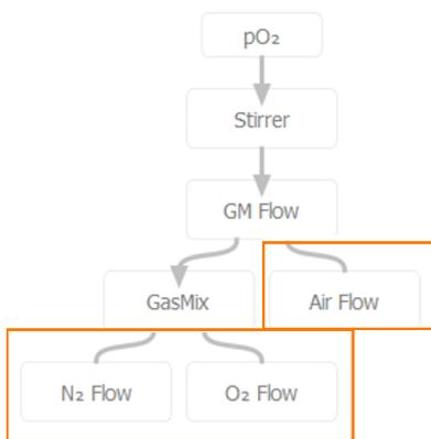
If both *O<sub>2</sub> Flow* and *N<sub>2</sub> Flow* are available, they will form a parallel cascade under the *GasMix* parameter.
