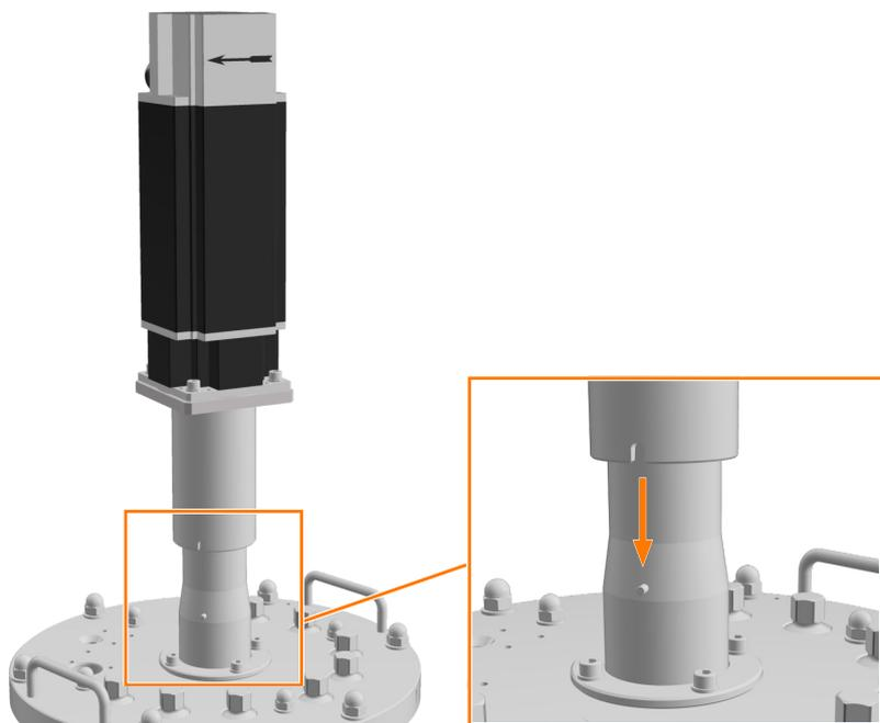
An air-cooled servo motor is used as drive. The motor is coupled by placing it on the drive hub on the vessel top plate. Here, the groove on the motor must be aligned with the pin on the drive hub. This locks the motor into its position.
