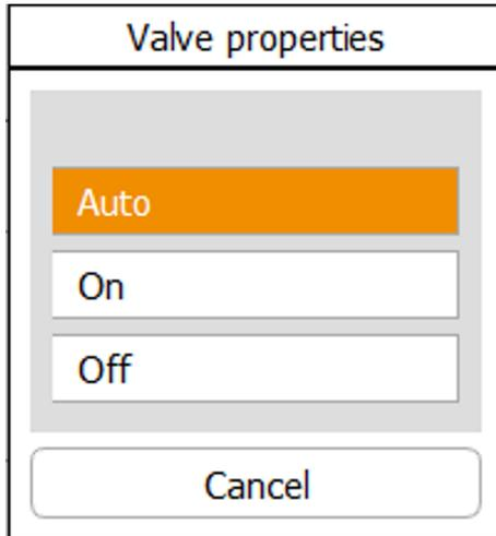
Pressing a valve button opens a dialog box where you can use **On**, **Off**, or **Auto** to change the valve status for diagnostic purposes.
