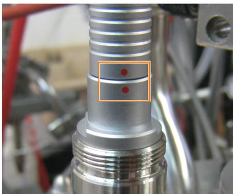
4. → Connect the sensor cable. In doing so, align the red marking of the cable plug with the red marking on the sensor head connection.
