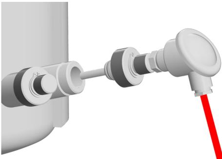
1. ➔ Insert the temperature sensor on the screw-in socket with O-ring in the Ingold nozzle.
