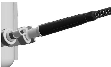
**3.** → If necessary, mount the cable kink protection according to the manufacturer's specifications prior to connecting the cable.
