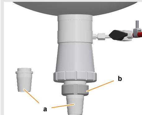
To harvest/empty, a valve insert with a nozzle (a) is used to connect the hose line provided by the operator. This is affixed using a groove nut (b).
