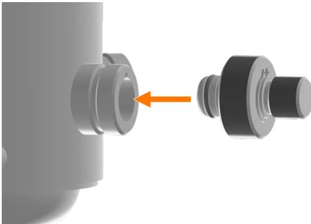
1. ➤ Insert the blanking plug with O-ring into the Ingold nozzle.
