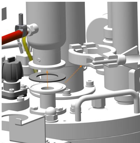
3. → Remove the clamp, exit gas cooler and flat gasket between the exit gas cooler and connection flange on the vessel top plate in the same way.
