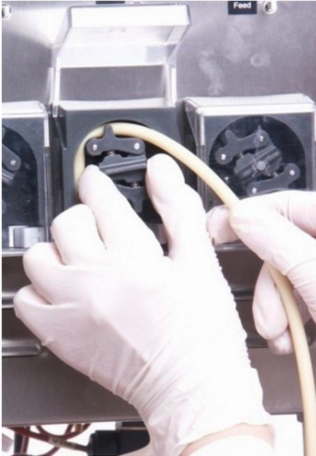
5. → Slowly turn the pump head clockwise with one hand and support the pump hose guide with the other hand.
