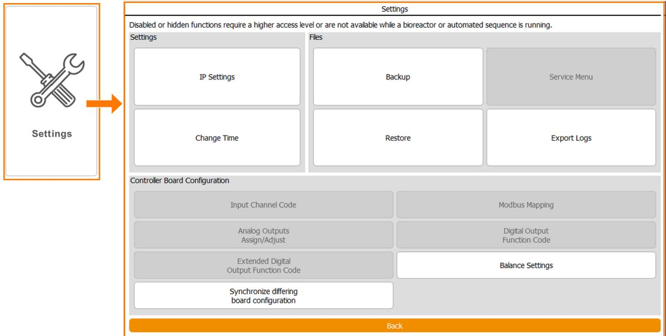
The basic settings of the device are made in the *Settings* submenu. The number of buttons visible and available in this menu depends on the authorisation of the user that is logged on. The figure above shows the menu for an *Administrator* user. The menu is divided into three sections with different functions.
