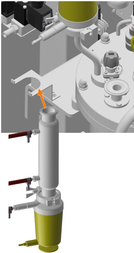
5. → Turn over the exit gas cooler and place it in the holder on the vessel mounting.
