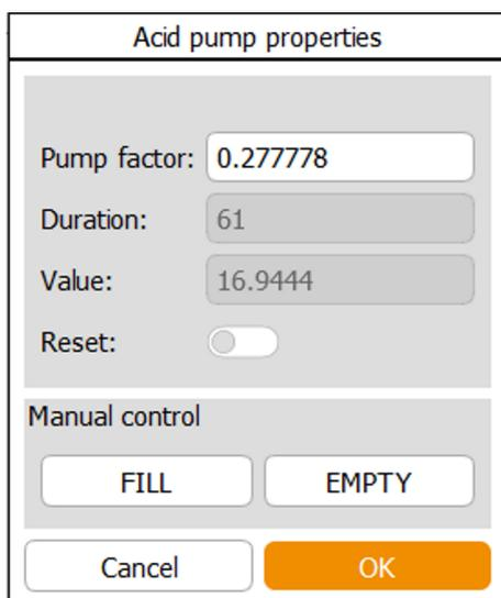
Pressing one of the pump buttons opens the *pump properties* dialog box of the selected pump in which the number of revolutions can be reset to zero. The pump factor calculated during a pump calibration is also shown here and can be changed manually. In addition, the **FILL** / **EMPTY** buttons enable manual filling or draining of the pump hose.
