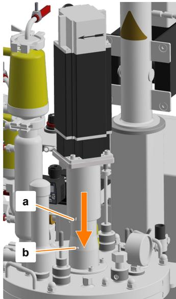
1. → Remove the motor from the holder on the central column or from the holder on the lifting device for the vessel top plate (if available).
