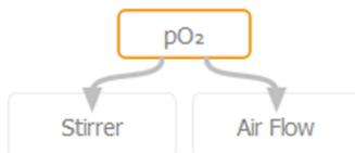
The parameters *Stirrer* and *Air Flow* are activated at the same time to control the  $pO_2$  parameter.
