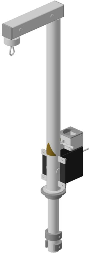
A lifting device is available for lifting and lowering the vessel top plate. This device is mounted on the central column of the basic unit and operated using a rope winch. We recommend using a lifting device in particular for vessels with a total volume of 30 liters and 42 liters.
