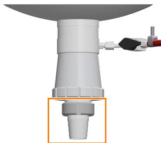
4. Attach the harvest hose to the nozzle of the harvest/sample valve or place the vessel underneath the harvest/sample valve.
