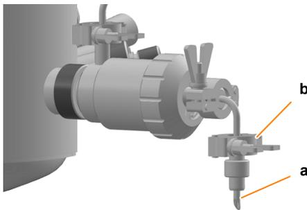
The sample valve has a needle (a) for sampling. The needle is connected to the condensate elbow (b) with a clamp and a flat gasket. For sampling, the steam trap must be unscrewed from the needle.
