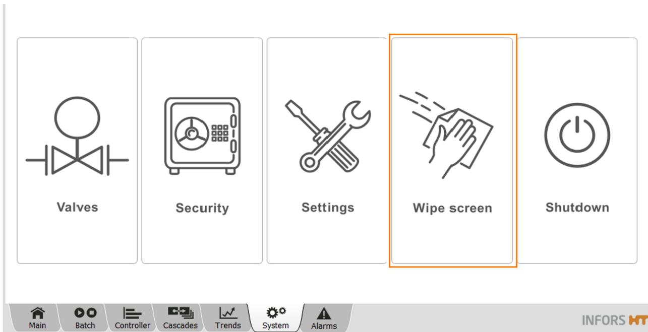
The *Wipe Screen* submenu has only one function: it locks all input on the screen for 20 seconds. This enables you to clean the screen within 20 seconds, if required.
