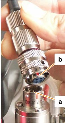
**METTLER analog, type InPro 6820/25/080 (amperometric, polarographic)**
