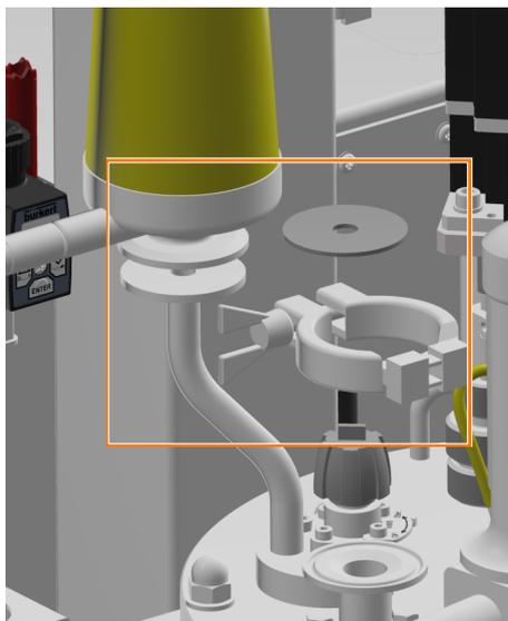
1. ➔ Place the flat gasket and flange of the inlet air filter flush on the flange of the vessel top plate.
