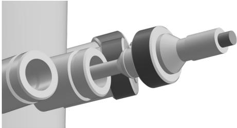
**2.** → Insert the sensor into the Ingold nozzles and tighten it manually using the coupling nut.
