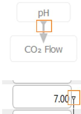
The fact that the Negative function is active is indicated by the triangle symbol on the arrow that indicates the direction of the cascade control.
