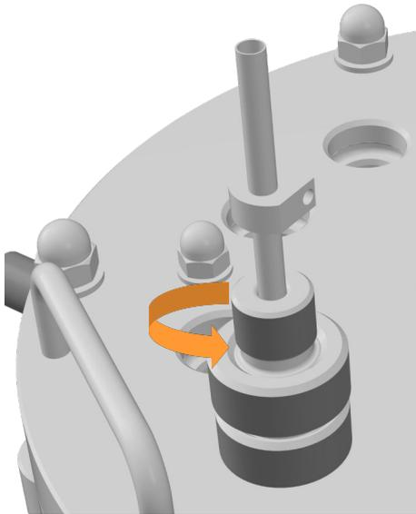
**4.** Carefully loosen the hollow screw by hand.
