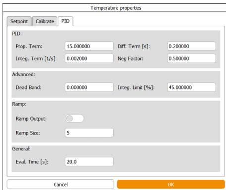
The *PID* menu contains input fields for setting up PID control (Proportional Integral Derivative control).
