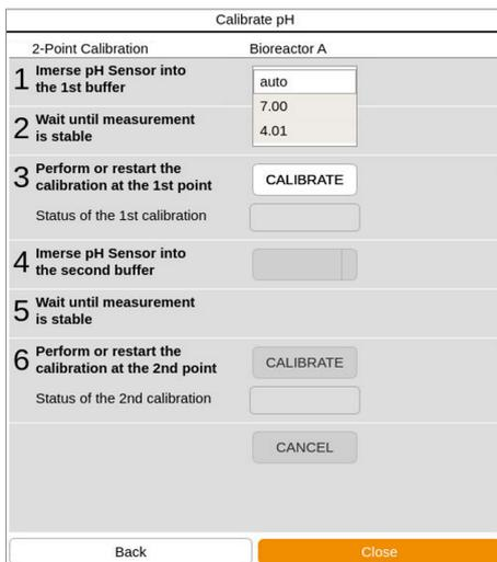
➔ The menu opens and guides you through the calibration step by step (1 to 6).
