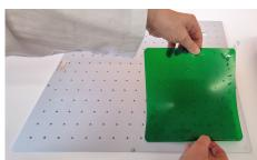
Apply the adhesive matting to the tray while still dripping wet. If there are cut-outs on the tray for fixing the tray, cover them. Do not cut out the adhesive matting under any circumstances.
