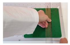
Gently run the ruler over the adhesive matting to remove the superfluous water and any air bubbles.
