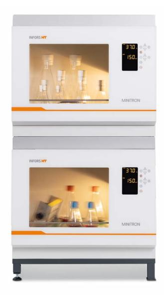
"Even with a maximum load with a culture volume totaling 7.5 L, the Minitron's low-vibration, quiet operation is impressive."
